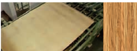
Boise Cascade peels the tree into veneers, with nearly all of the wood fiber going to structural "best" use.
