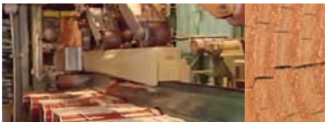
Dimension lumber cuts the heart out of the tree, with only about 60% of the tree going to structural "best" use.
