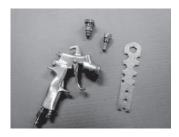
7. Flush the gun with water. Use a soft-bristle brush to clean out any remaining stain or buildup within the gun.
