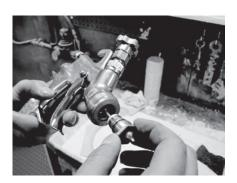
4. Unscrew the needle adjustment knob from the back of the gun and pull out the needle.
