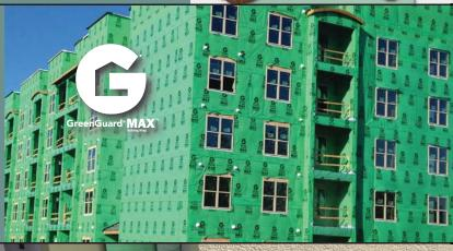
GreenGuard® MAX™Building Wrap is a recognized air barrier listed with www. airbarrier.org, and has demonstrated water holdout capabilities in industry-recognized water resistance tests. This non-perforated wrap also breathes to allow moisture vapor to escape. With its high tear resistance, it is suitable for commercial and residential applications. It remains UV stable up to 6 months.
