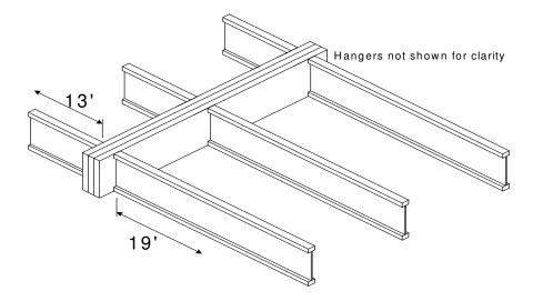
Find: A multiple 1 3/4" ply VERSA-LAM that is adequate to support the design loads and the member's proper connection schedule with Simpson SDW screws.
